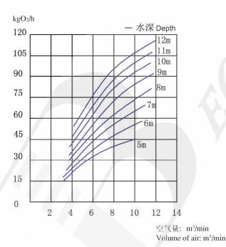
QSB15溶氧性能曲线 Curve of oxygen-dissolving performance for QSB15
